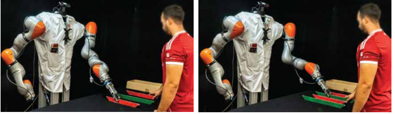
Figure 8: Physical deployment of the evolved DNF controller in the collaborative packaging task. To the left, the complementary response : the workspace contains two small red frames and one large green frame. The human grasps the right small frame, and the robot independently selects the left small frame. To the right, the cooperative response : the workspace contains two large green and two small red frames. The human grasps the left large frame, and the robot coordinates by grasping the same object.
